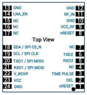
Figure 3-2 Pin Assignment
