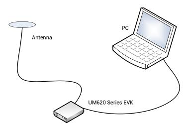
Figure 2-1 Typical Installation of UM620 Series EVK
