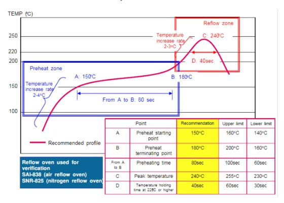
Figure 6-1 Reflow Soldering Temperature Curve
