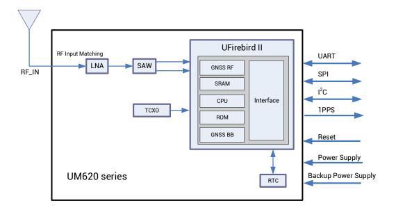
Figure 1-2 UM620 Series Modules Block Diagram
